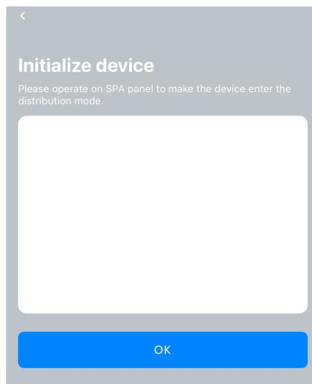
Go to the setting interface of the control panel, and stop the cursor at the WiFi option. At this time, press the confirm button on the panel to set the WiFi to AP. After setting, click OK on the app.
